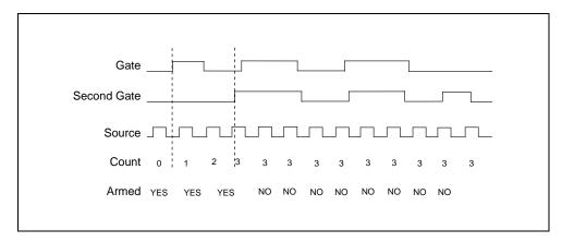
Figure 2-18. Start-Stop Measurement
